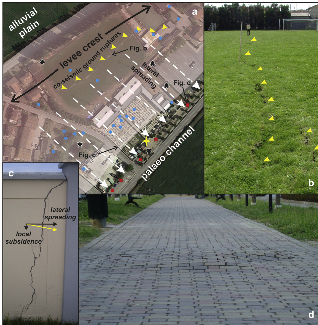
Fig. 8. Geomorphological features observed in Mirabello the area (see Fig. 2 for location): a) Google Earth frame of the cemetery area showing the distribution of secondary co-seismic effects, such as sand ejection points (blue dots), ground deformation sites (red squares), drill cores (black stars), ground ruptures (yellow arrows) and sliding direction due to lateral spreading (white arrows). The yellow star indicates the location of benchmark 78020 characterized by 11.4 cm of subsidence. b) Ground ruptures observed on top of the abandoned levee (see (a) for location). c) Effects of the lateral spreading on the lateral wall of the cemetery (see (a) for location). d) Example of ground deformation associated with shallow liquefaction (see (a) for location). (For interpretation of the references to color in this figure legend, the reader is referred to the web version of this article.)
